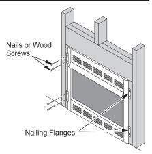
Figure 17 - Attaching Fireplace to Wall Studs
